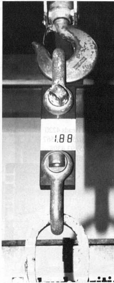
Only two shackles are required to fit the Dynafor load indicator into the lifting arrangement.
