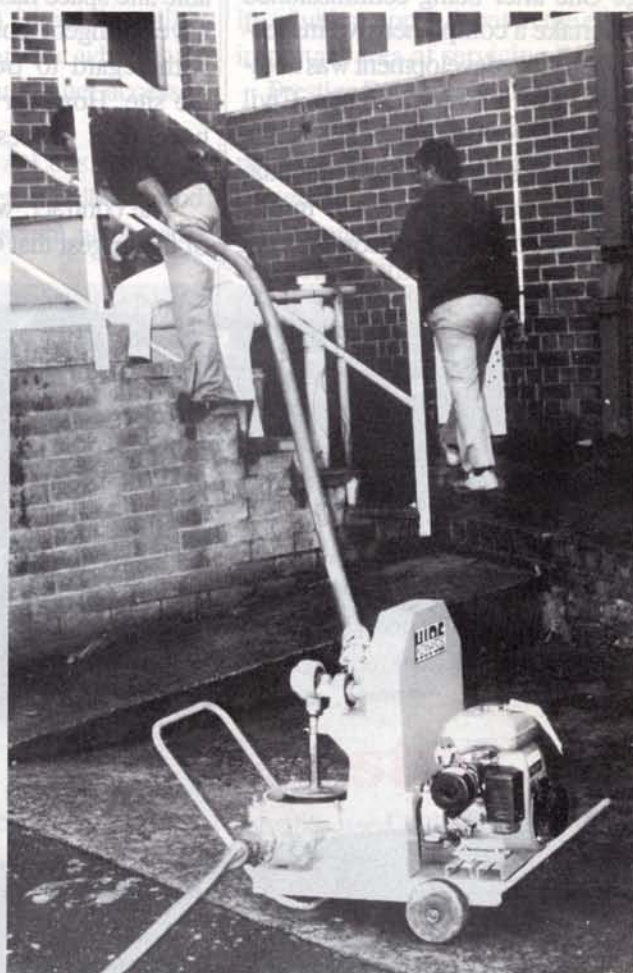
A diaphragm pump from Kennards Hire empties a settlement tank at a major Sydney Hospital.
