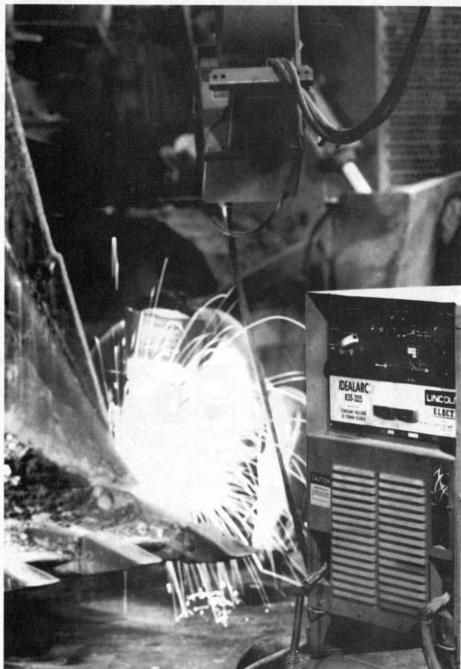
A welding engineer repairing the worn out outer section of a dozer bucket using Lincoln Electric's new flux cored hardfacing wire giving quick and quality deposition of weld material
